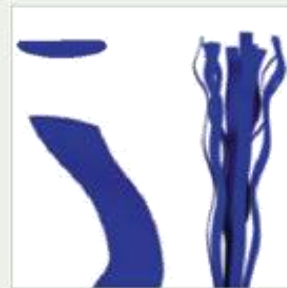
Fibre thickness: approx. 110 µm
